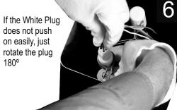
While holding the SAME side of the Lamp attached to the clamp, carefully push on the white plug. NOTE: Although the Lamp is fairly strong, too much tension from the opposing side may break the Lamp.
